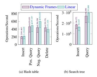
Figure 7: Median throughput of subcomponent microbenchmarks. Higher is better. Error bars are min/max of 6 runs.
