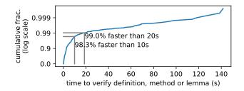
Figure 4: Cumulative distribution of verification times of function definitions, implementation methods, and proof lemmas. Most definitions–99.0%–verify in less than 20s, and 98.3%– verify in less than 10s.
