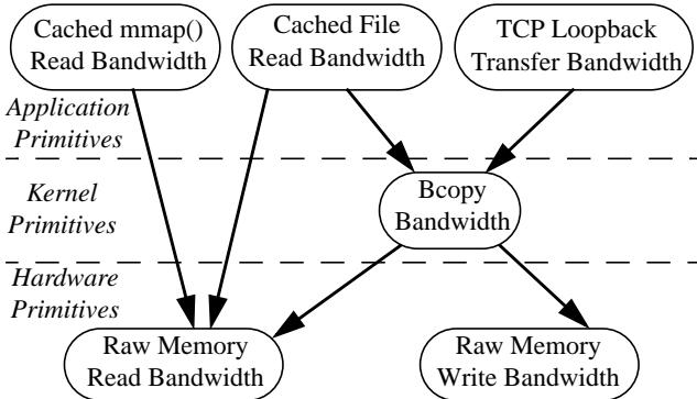
**Figure 2: Decomposition of Application Data-access Primitives.** All of the application-level data primitives for bulk data access depend on the hardware’s memory read bandwidth since they all touch data. File reading interposes the extra overhead of a cross-protection-domain bcopy to move the requested data to user-space buffers; TCP transfer interposes three bcopy’s as it shuffles the data through the loopback interface and between user and kernel space.
