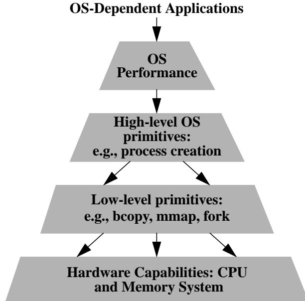
**Figure 1: Decomposition of OS performance via *hbench:OS* primitives.** The performance of OS-dependent applications (such as web servers) can be decomposed into high-level OS-provided services and primitives, which can in turn be decomposed into low-level kernel primitives, which can again be decomposed into hardware capabilities. In many cases, *hbench:OS*'s suite of tests allows us to measure and relate the lower three levels of this hierarchy.
