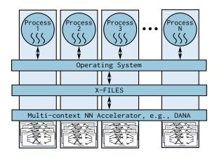
Figure 1. A multiprocessing system has processes composed of threads managed by an operating system. We propose a set of hardware/software extensions, the X-FILES, that enable the multi-context management of requests by processes to execute NNs in their respective address spaces on an underlying NN accelerator.
