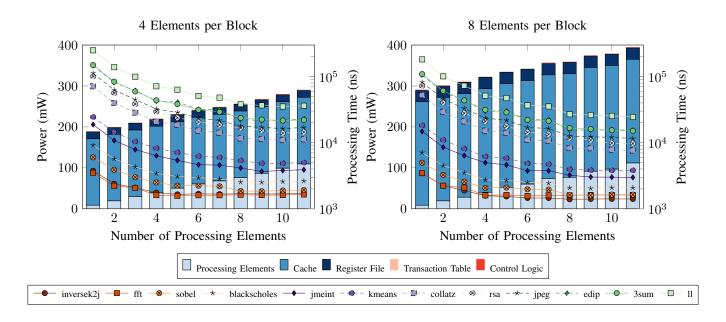
Figure 10. Average power per module (bar plot) and processing time (line plot) of different NN configurations, listed in Table III, when running exclusively (i.e., one NN at a time) on DANA architectures with 1–11 processing elements and four or eight elements per block.
