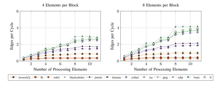
Figure 11. DANA's throughput, measured in edges per cycle, when executing one instance of an NN transaction.
