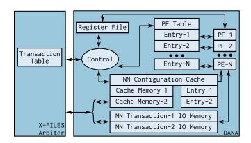
Figure 6. Architecture of DANA. Control logic dynamically allocates processing elements to neurons of executing NN transactions read from the X-FILES arbiter. Inputs and outputs are stored in per-transaction memories, NN configurations are stored in a local cache, and intermediate computations are stored in a Register File.
