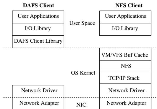
Figure 1: User-level vs. kernel-based client file system structure.
