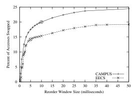
Figure 1: The effect of different window sizes on the percentage of swapped accesses. The sorting window size chosen for each host is shown with a circle: for EECS, 5ms is sufficient, but for CAMPUS 10ms is better.
