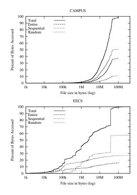
Figure 2: Percentage of bytes accessed randomly, sequentially, or in their entirety verses the total bytes accessed. Each run is categorized according to its access pattern and then all of the bytes accessed in this run are added to the subtotal for this category. These runs are computed by the heuristic described in Section 4.2.
